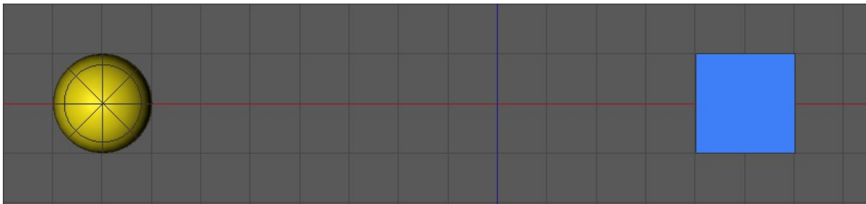
Figure 11 – after mirroring using global coordinates, the sphere is at global X -800 (-1300 local)
